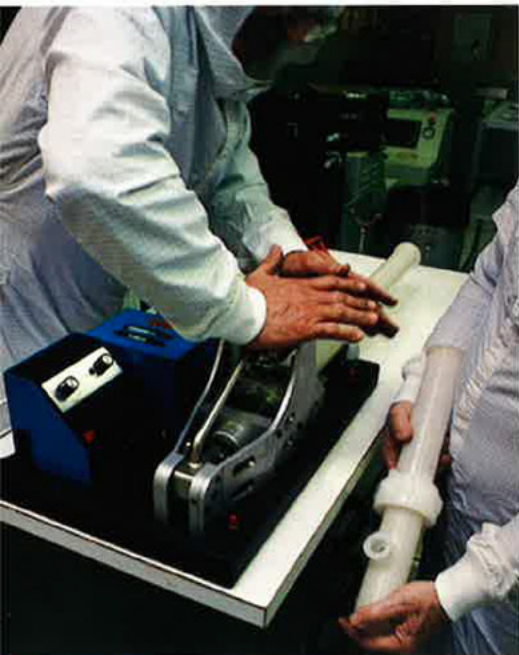
KYNAR PVDF piping is ideally suited to on-site fabrication, reducing the risk of contamination and speeding the installation process.
