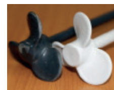
(left) worn epoxy coated impeller (right) Rilsan® PA11 coated impeller
