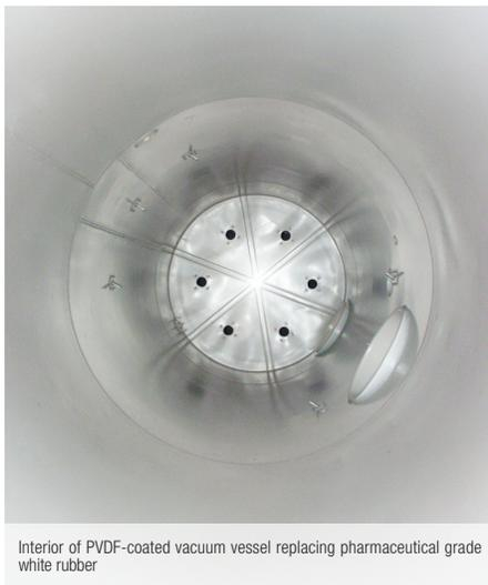
Interior of PVDF-coated vacuum vessel replacing pharmaceutical grade white rubber
