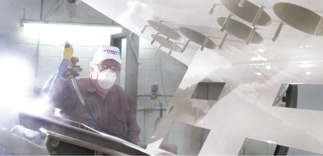
Figure 5. Application of electrostatically sprayed PVDF powder coatings. Graphic courtesy of Fisher Company
