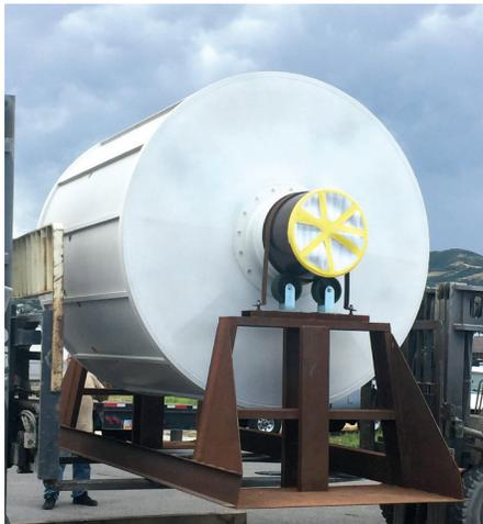
Rotary drum filter coated with PVDF replacing FRP and elastomeric linings. Service is elevated dilute HCl and organics.
