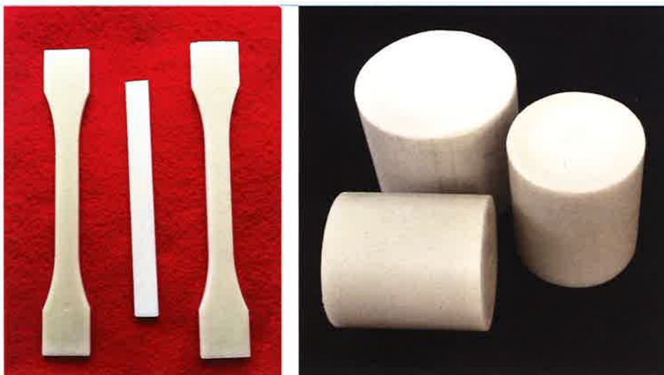
Glass-reinforced compounds are made with Kynar UHM resin of relatively high MFR so they can be injection molded at temperatures below 210 C (410 F) and extruded at or below 240 C (464 F).
