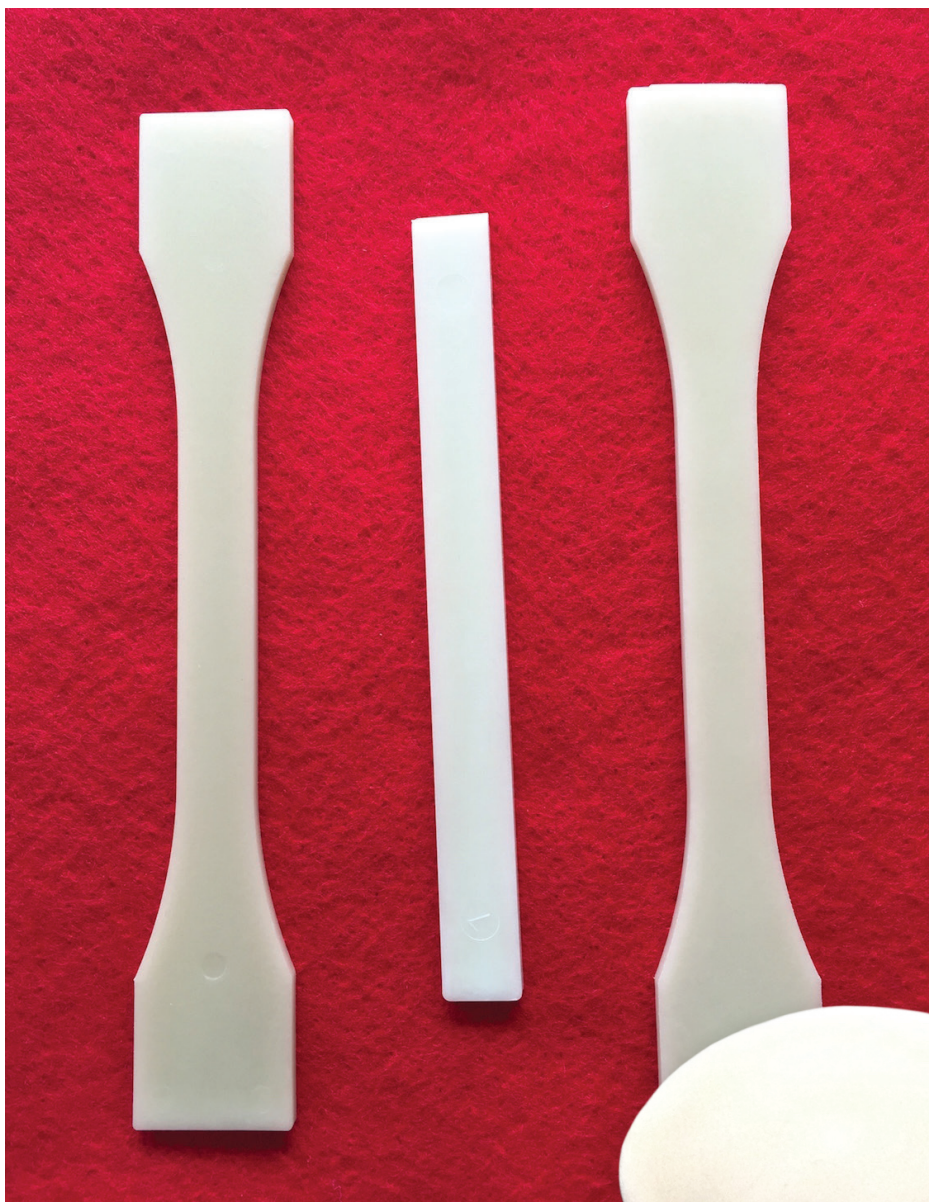
Image 2. Injection-molded tensile bars made with glass-reinforced PVDF
