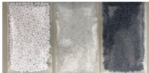
Figure 1. Three recycled polyethylene resin samples provided by Polykar from left to right: white, natural, gray.
