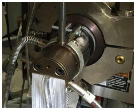
Figure 2. The flat die extruder used for the melt fracture elimination and melt pressure reduction studies.
