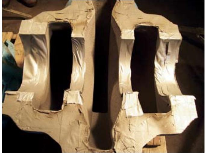
Figure 6. Denise No. 2 horizontal split-case pump – upper half of pump housing after masking the seal areas and grit blast cleaning.
