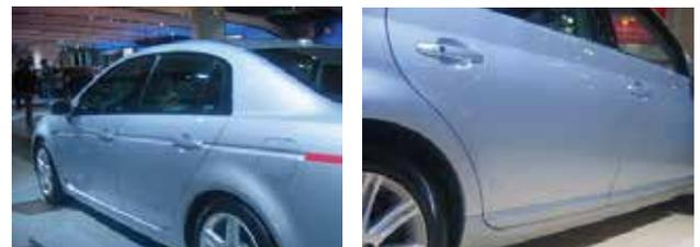
*Kynar® fluoropolymer films provide an attractive, corrosion-resistant alternative to paint.*
