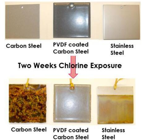
Figure 4. Kynar Flex PVDF coatings versus metal in two weeks of chlorine exposure. Graphic courtesy of Arkema
