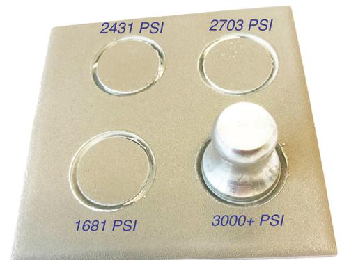
Figure 6. Adhesion testing of PVDF coatings bonded to metal substrate. Graphic courtesy of Fisher Company
