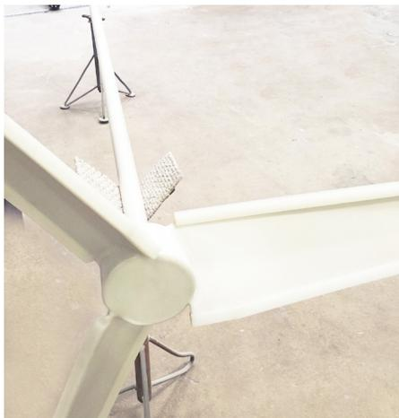
PVDF electrostatically applied coating with welded PVDF edge protectors. This mixer replaced rubber-lined steel in a highly abrasive and low pH mineral process application.
