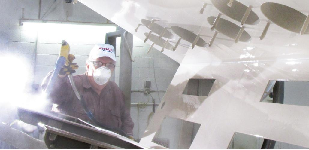
Figure 5. Application of electrostatically sprayed PVDF powder coatings. Graphic courtesy of Fisher Company
