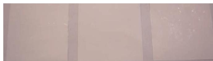
**Figure 5: Kynar® PVDF Membranes after Exposure to Cleaning Chemicals**
