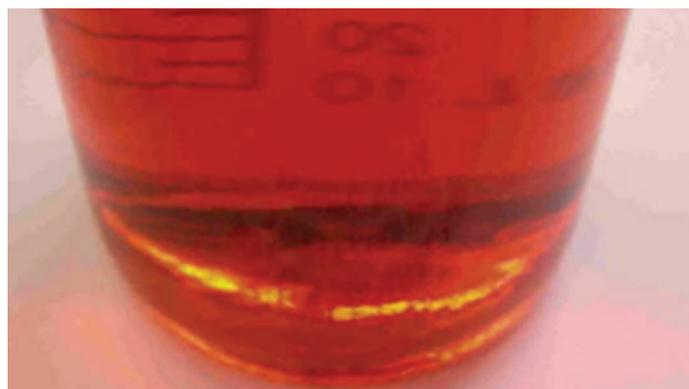
**Figure 2: Nylon (PA 6,6) Membrane after Exposure to Bromine Water**
