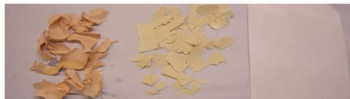
**Figure 4: Polysulfone Membranes after Exposure to Cleaning Chemicals**
