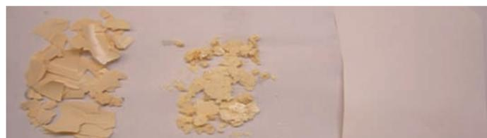
**Figure 3: Polyethersulfone Membranes after Exposure to Cleaning Chemicals**
